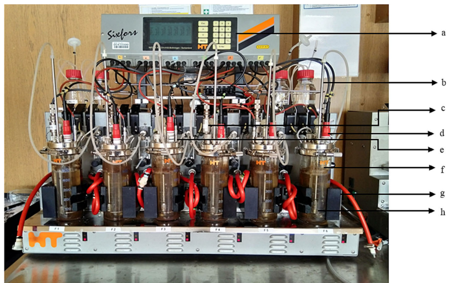
FIGURE 2 Laboratory-scale SIXFORS plant (Infors® HT): (a) U-DDC control panel and display, (b) inlet of aeration unit, (c) dissolved oxygen sensor, (d) pH sensor, (e) temperature sensor, (f) reactor containing deammonifying sludge of MWWTP Kaster, (g) thermostat, (h) air diffuser.
