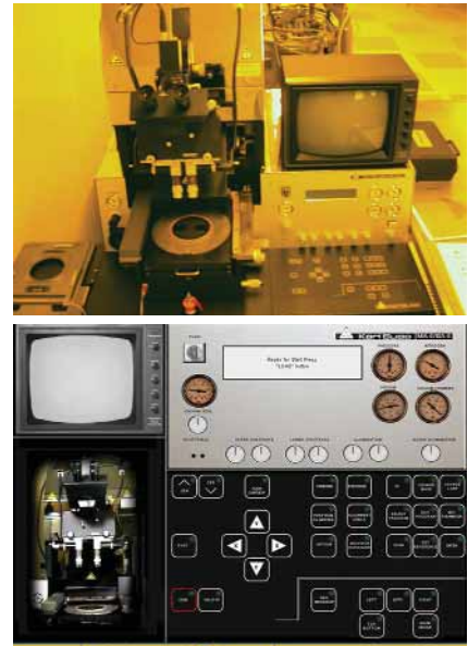
Figure 3: The real mask aligner MA6 and its virtual pendant, i.e. the computer-based training tool.
