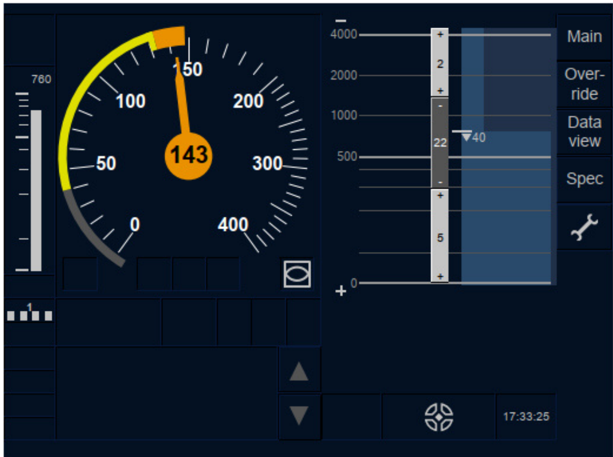
Bild 2-5 Driver Machine Interface [ERA_ERTMS]
