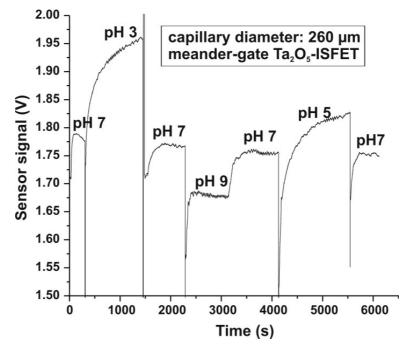
**Figure 7.** Constant-charge-mode dynamic response of a meander-shaped  $Ta_2O_5$ -ISFET (layout (a) in Figure 5) in buffer solutions of different pH values from pH 3 to pH 9 measured at wafer level by means of the developed experimental set-up with the micro-droplet cell.
