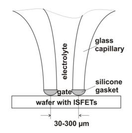
**Figure 2.** Capillary microcell for spatially resolved electrochemical measurements on wafer level. A silicone gasket at the tip of the capillary defines the testing area.
