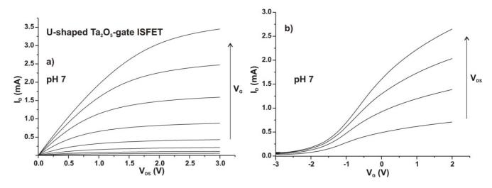
**Figure 6.** Output (a) and transfer (b) characteristics of an ISFET (layout (b) in Figure 5) measured on wafer level by means of the developed experimental set-up with the micro-droplet cell.
