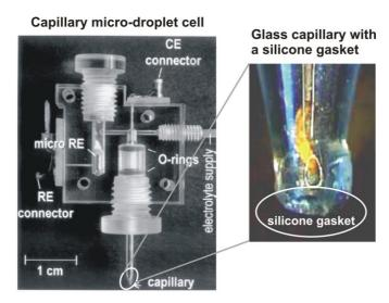
**Figure 4.** Capillary micro-droplet cell for testing of ISFETs on wafer level (RE: reference electrode, CE: counter electrode).
