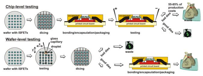
Figure 1. Wafer-level vs. chip-level testing.
