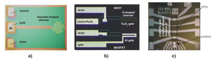
**Figure 5.** Layouts of different ISFET chips consisting of a single ISFET with a meander-shaped channel (a), an ISFET/MOSFET (metal-oxide-semiconductor FET) pair with an U-shaped channel (b) and four ISFETs and one MOSFET with a linear-shaped channel (c).
