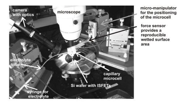
Figure 3. Photo of the ISFETs' wafer-level testing system.
