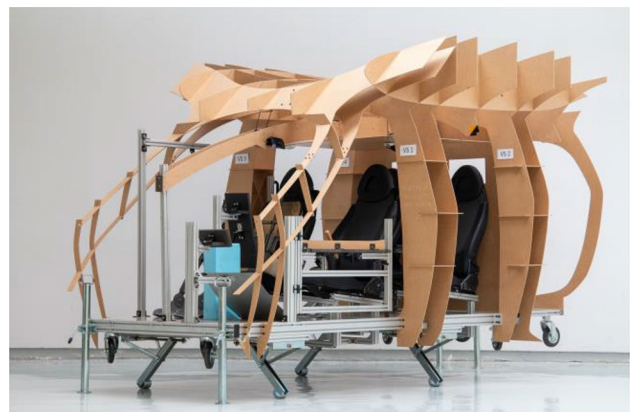
Fig. 3 Seat box of SkyCab eVTOL
