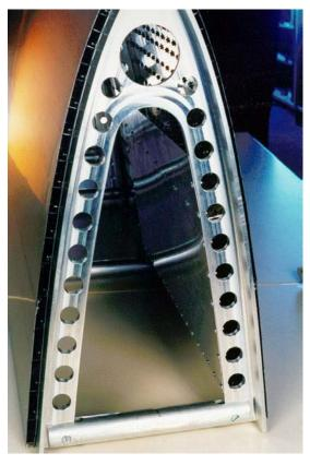
Figure 4: RaWid manufacturing concept for suction noses
