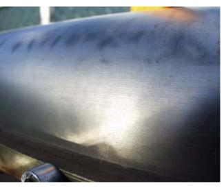
Figure 8: Titanium skin with holes (test chamber)
