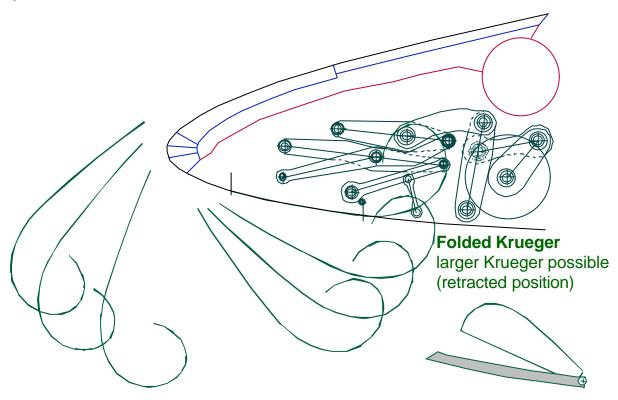
Figure 2: Space allocation study of a hybrid laminar wing nose for a MEGALINER
