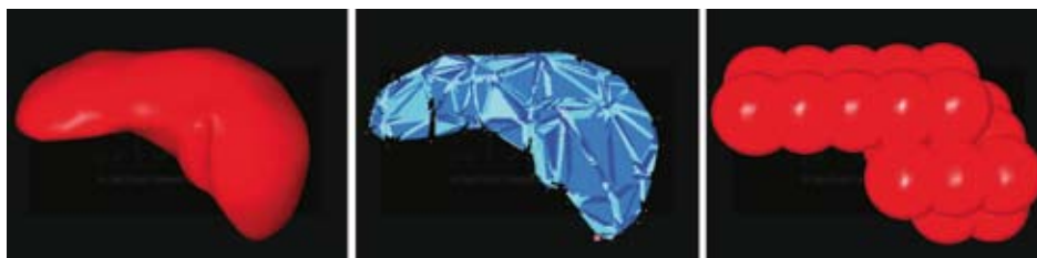
Fig. 1 | Liver in SOFA: visual model, mechanical model, collision model, respectively, [3].
