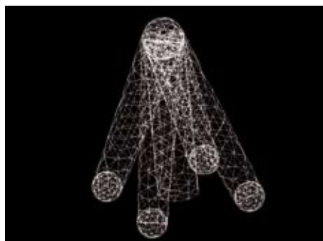
Figure 2 | A discretized model of the anchor.
