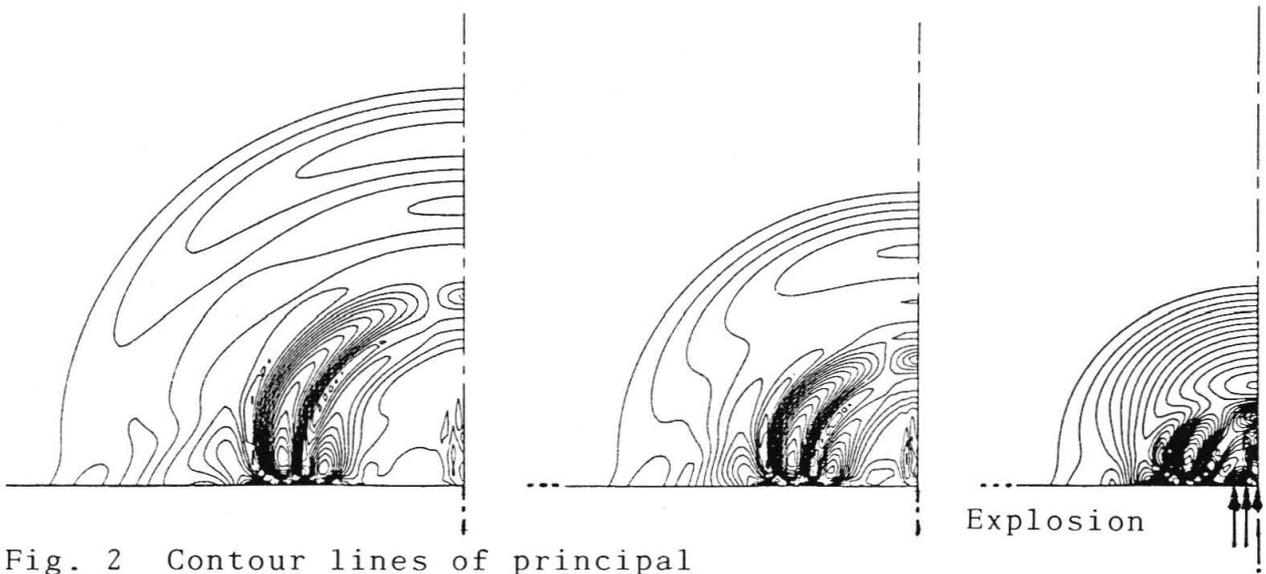
Fig. 2 Contour lines of principal shear stresses
