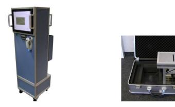
*Figure 4: Prototypes of plant scanners. Right: Phytoscan alpha 70, for green house studies (battery, internet, USB), Left: Mobile scanner prototype for field studies portable in a suitcase.*
