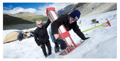
Figure 1. Testing of the IceMole prototype on the Morteratsch glacier.
