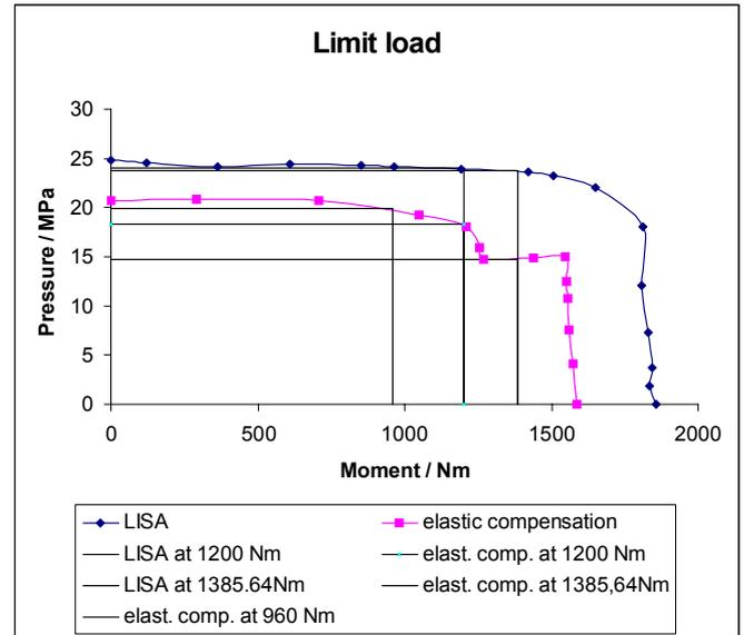
Fig.2: Limit load interaction diagram for thick-walled cylinder–cylinder intersection.
