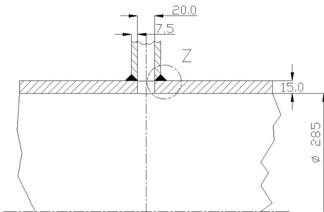
Fig. 1: Thick-walled cylinder–cylinder intersection.
