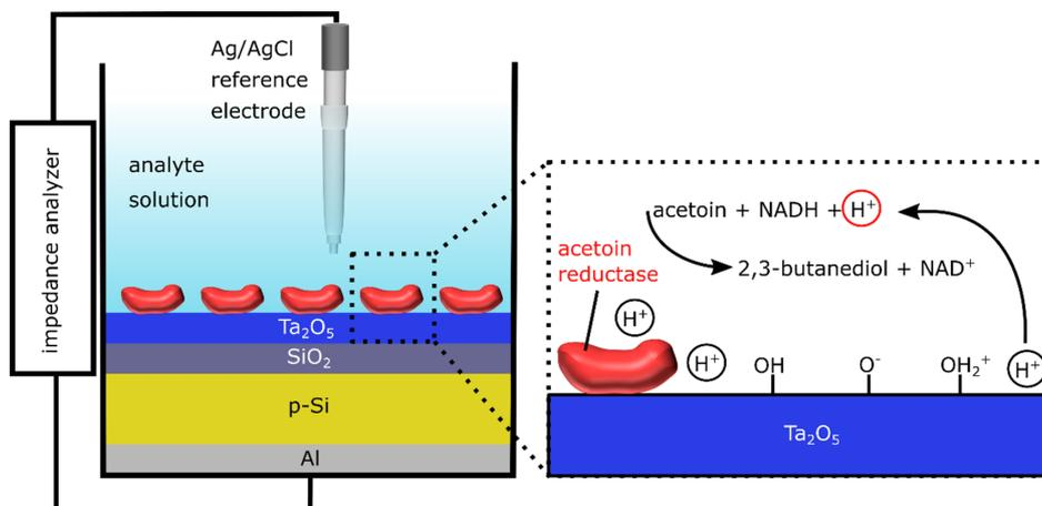
**Figure 1.** Schematic layer structure of the Al/p-Si/SiO<sub>2</sub>/Ta<sub>2</sub>O<sub>5</sub>-enzyme EIS sensor with measurement setup (left), and enzymatic reduction of acetoin catalyzed by the enzyme acetoin reductase (right).
