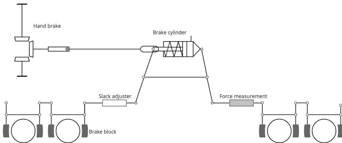
**Fig. 4** Instrumented brake rigging
