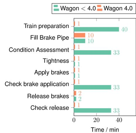
Fig. 8 Time consumed for the individual steps of brake tests, existing fleet (Wagon < 40) compared to Wagon 4.0
