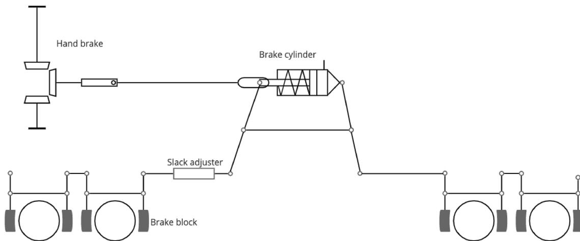
**Fig. 3** Braking force generation
