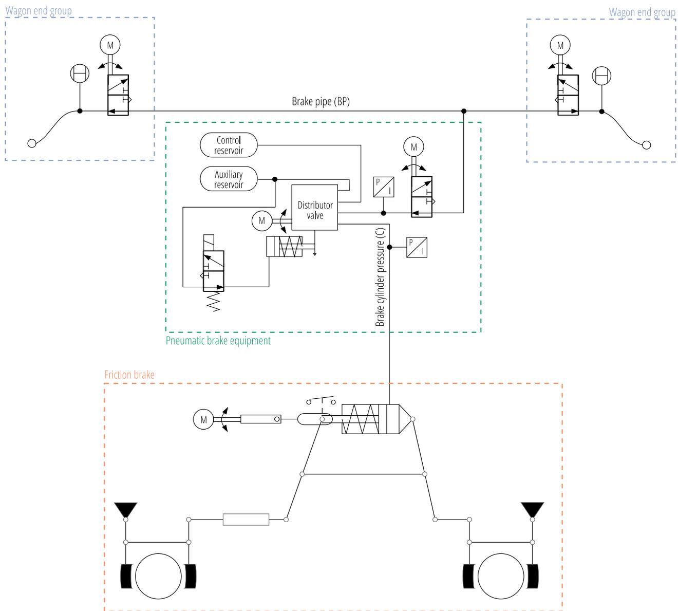
**Fig. 7** Automated pneumatic brake schematic for Wagon 4.0
