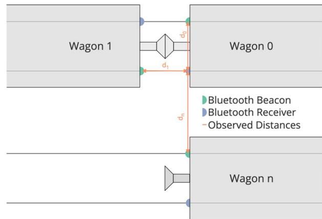
**Fig. 6** Connection example: wagons 0 and 1 form a rake, wagon n would lead to a false detection
