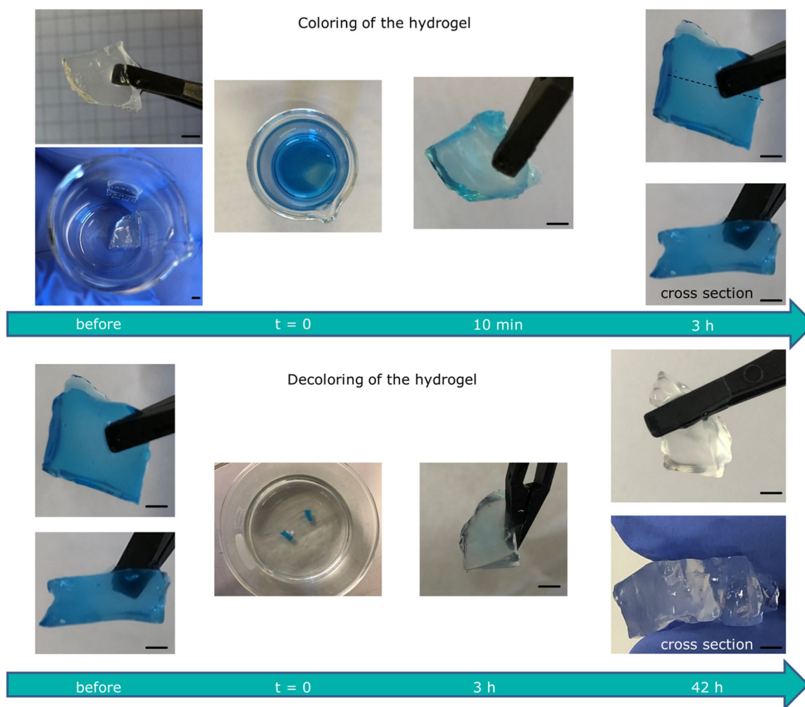
FIGURE 9 Dyeing a piece of hydrogel with cresyl-blue staining solution for 3 h (top row). The piece of hydrogel was cut in half to prove the uniformly stained cross section. Bleaching of the hydrogel by using deionized water (bottom row). After 42 h, no visible sign of the stain remained. The scale bar equals 2 mm.
