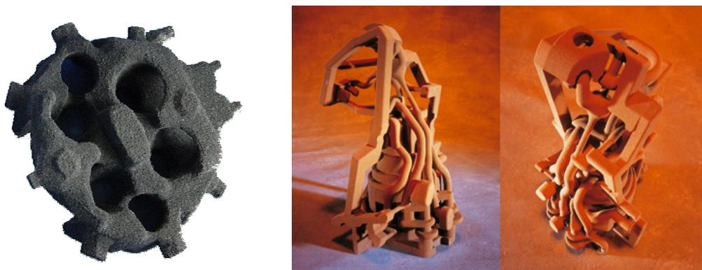
**Figure 6:** Generative fabricated Kernels for Metal Casting. 3D-Printig (ProMetal, left)
