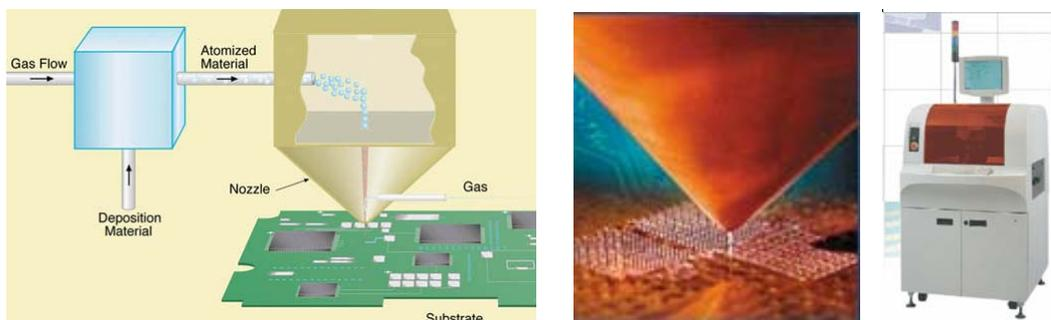
**Figure 12:** Maskless Mesoscale Materials ( $M^3D$ ) Process, Optomec. Process Scheme (left), Aerosol Printing Head (middle), Machine (right).
