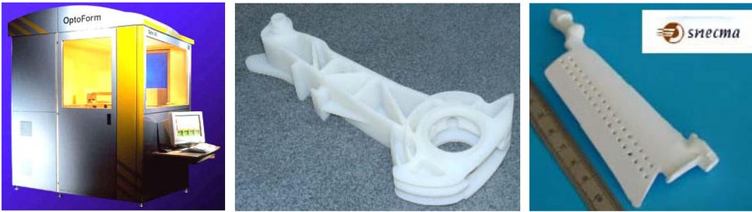
**Figure 10:** Stereolithography, Paste Polymerization. Machine (left), part and Turbine Blade made from Ceramics. (3D Systems-DSM Desotech /Optoform LLC)
