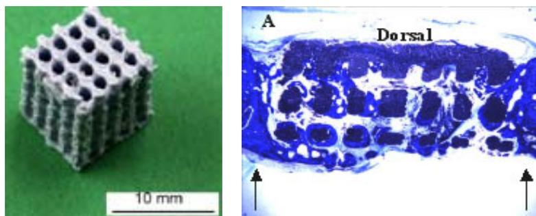
**Figure 5:** Demo Part with guiding Channels made from artificial Bone Material, 3D Printing (FORTEPRO, left), New Bone Material (blue/grey), grown in the guiding Channels (light grey/ white) of the new Bone Structure (blau/grey), (THERICS, right)
