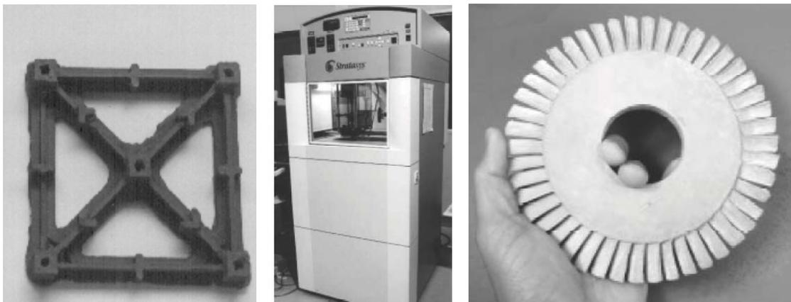
**Figure 2:** MJS Part made from silicon carbide (SiC) made by IFAM, IPA, left. FDC Machine (middle), EFF Part (right).
