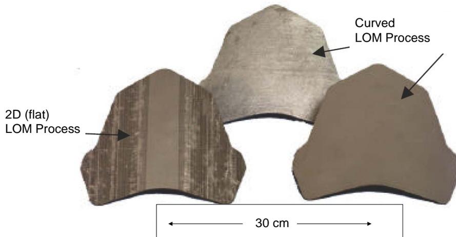
**Figure 9:** Layer Laminated Part. Flat LOM Process with Stairstepping (approx. 90 \* 90 \* 18mm, left); spatial curved LLM Part (middle and right). All Parts are made from SiC [KLO99].
