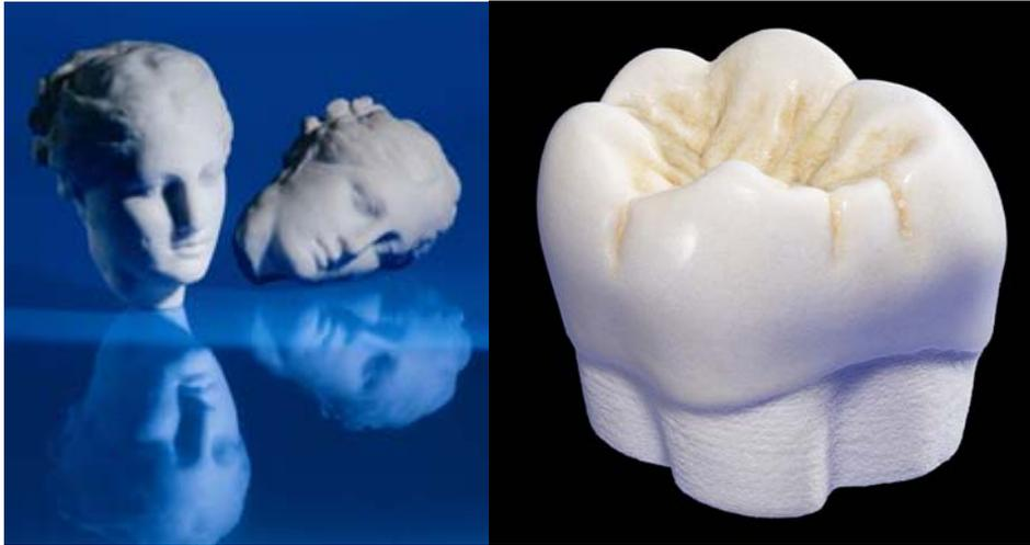
**Figure 3:** Sculpture, 3D Printing. Head of the Hygieia, Goddess of Health. Polished Marble Powder. (ProMetal, IFAM Bremen, left), Model of a tooth, Plaster-Ceramic (Z-Corp, RP Lab Aachen University of Applied Sciences, right)
