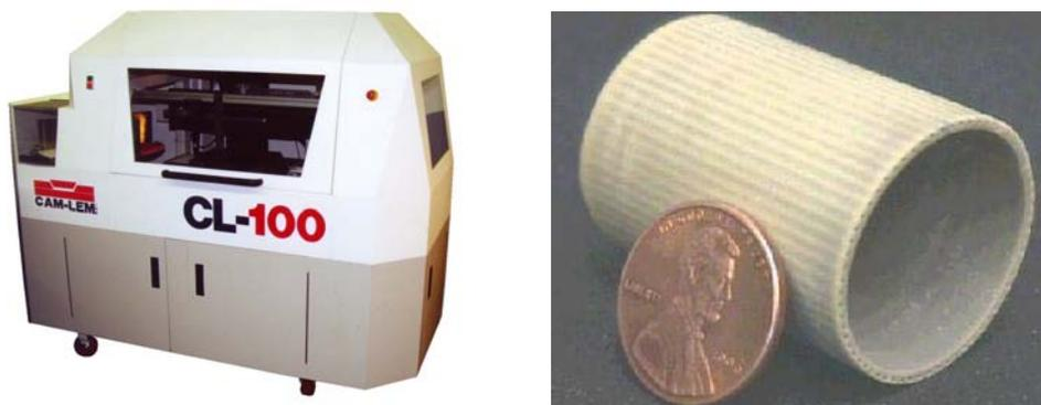
**Figure 8:** CamLem Process. Machine CL-100 (left); Cylinder with integrated Cooling Channels (right).
