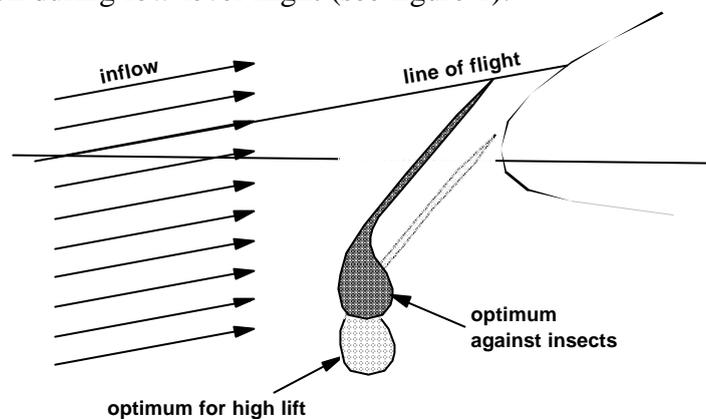
Figure 1: Krueger flap for insect protection
