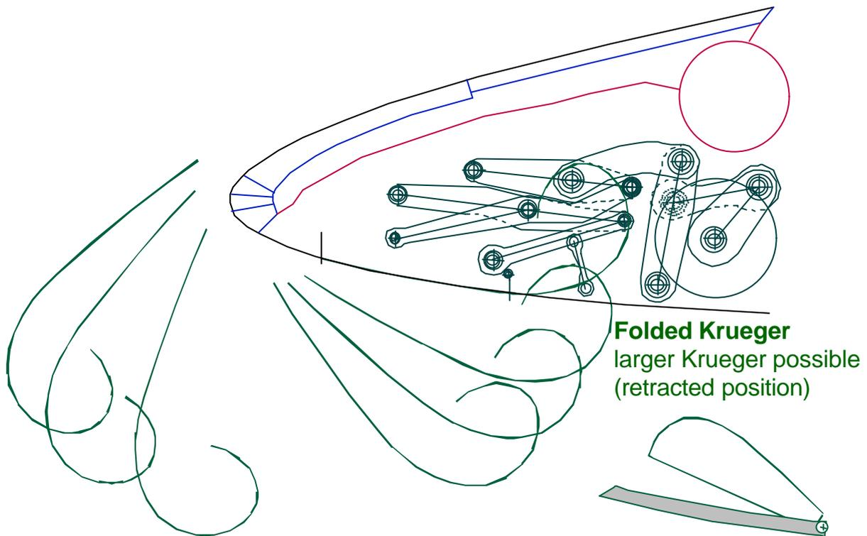
Figure 2: Space allocation study of a hybrid laminar wing nose for a MEGALINER
