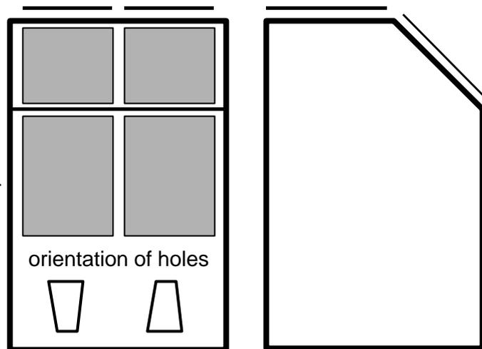
Figure 6: Ground test rack for perforated plates
