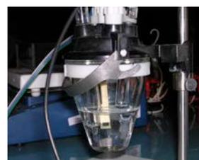
Figure 2: Impedance spectroscopy set-up
