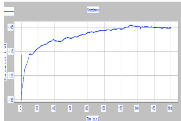
Figure 2. curve stabilization of the corrosion potential versus time for Al-40 wt % Mg alloy
