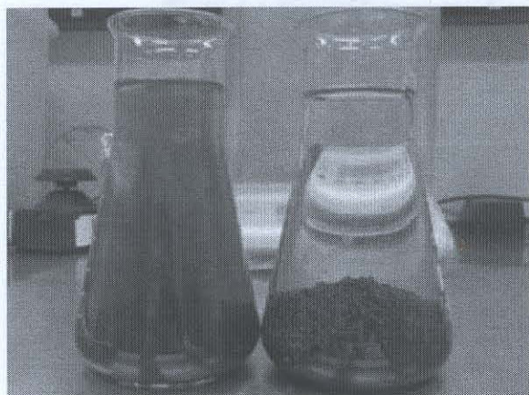
Fig. 4. Left: Highly dispersed fraction (dust) removal from the sample has succeeded after 3 washing steps. Right: Autoclaving of the material removes air from the pores and significantly enhances adsorption capability. After autoclaving, material sediments since it has higher density than water.
