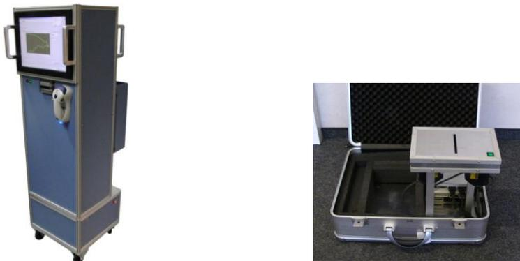
Figure 4: Prototypes of plant scanners. Right: Phytoscan alpha 70, for green house studies (battery, internet, USB), Left: Mobile scanner prototype for field studies portable in a suitcase.
