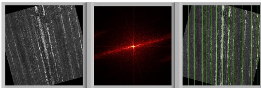
Figure 3: Same leaf as above inclined to the Laser line by  $15^\circ$ . Left: inclined original. Middle: 2D Fourier transformation, right: for orientation corrected image of the leaf with bundles (green).
