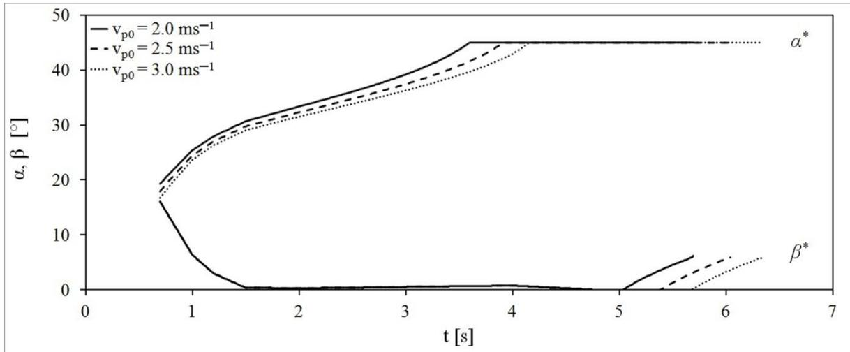
**Figure 4:** Optimized time courses  $\alpha^*(t)$  and  $\beta^*(t)$  for various  $v_{p0}$  on the HS 205 m ski flying hill.
