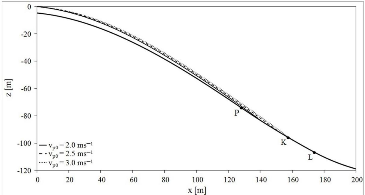
**Figure 3:** Flight paths of flight styles optimized for various  $v_{p0}$  on the HS 205 m ski flying hill. P-Point: 148 m, K-Point: 185 m, L-Point (HS): 205 m.
