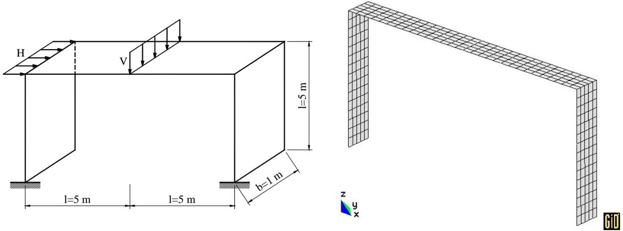
**Figure 2:** Geometrical dimensions and FE-mesh of the frame
