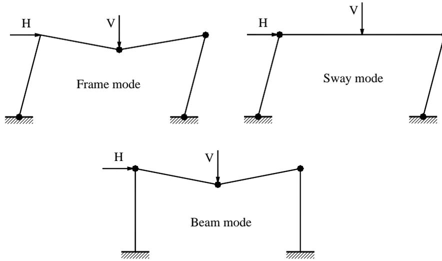
**Figure 3:** Three failure modes of the frame
