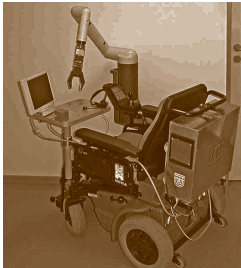
Fig. 53.4 Wheelchair manipulator robot MANUS developed at the Rehabilitation R&D Center, Hoensbroek, and marketed by Exact Dynamics (The Netherlands)
