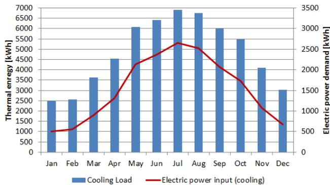
Figure 3-1: Cooling load of the reference building and electricity consumption of the air-conditioning as monthly sums
