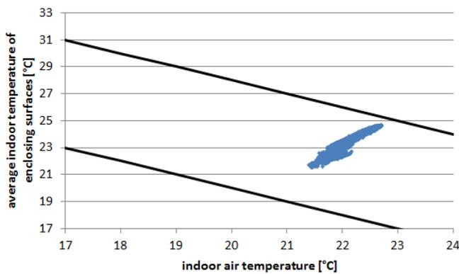
Figure 5-2: Average temperature of enclosing surfaces (simulation) in dependence of the room air temperature for the period of a year
