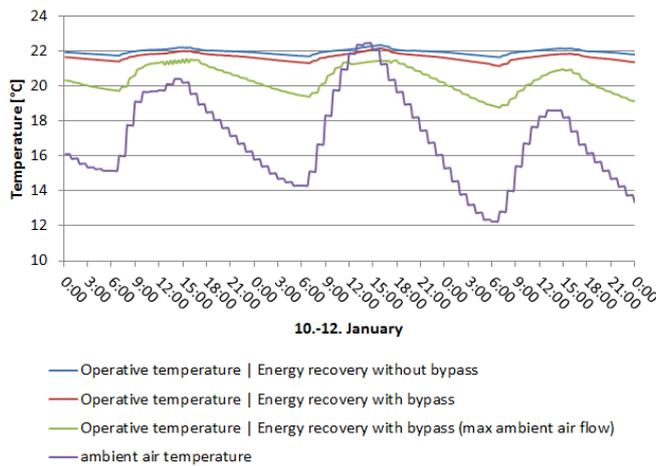
Figure 4-4: Trend of operative interior temperature for ventilation without bypass (blue), ventilation with bypass (red) and ventilation with bypass (max. outside air flow) as well as the ambient air temperature (purple) for three characteristic days in January
