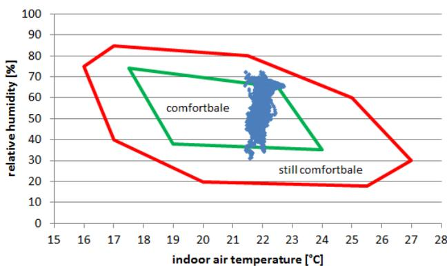
Figure 5-3: Relative air humidity in the interior (Simulation) in dependence of the room air temperature
