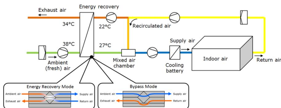
Figure 4-1: Simplified scheme of the ventilating system of the Passivhaus-Villa
