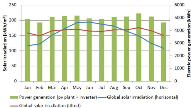
Figure 2-4: Monthly electric power production of the photovoltaic system on the roof of the Passivhaus-Villa (green) and monthly sums of the global solar irradiation into the horizontal (blue) and the module-pane (red) (module inclination: 35°, module orientation: 155°).
