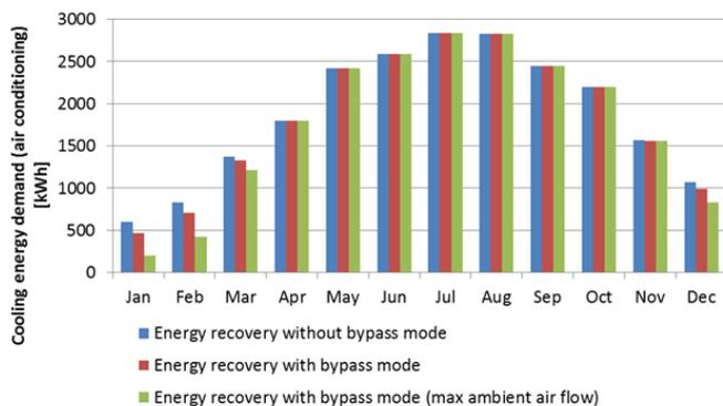
Figure 4-2: Energy demand of the ventilating system for the conditioning of the supply air for operating states without and with activated bypass function of the energy recovery system
