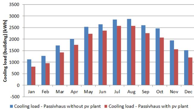
Figure 2-3: Cooling load of Passivhaus-Villa without (blue) und with PV installation (red)
