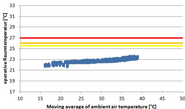
Figure 5-1: Image of the operative room temperature (Simulation) in dependence of the moving average of the ambient air temperature for the period of a year
