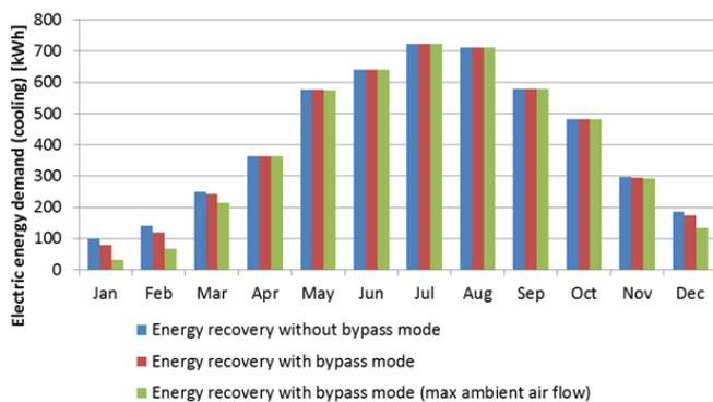
Figure 4-3: Electric energy demand of the ventilating system for operating states without and with activated bypass function of the energy recovery system
