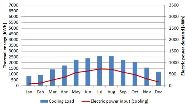
Figure 3-2: Cooling load of Passivhaus-Villa and electricity consumption of the air-conditioning as monthly sums
