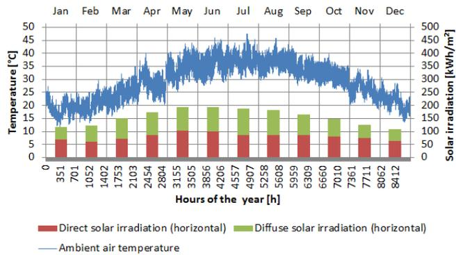
Figure 2-1: Ambient air temperature and solar irradiation (direct- / diffuse-horizontal) at the location of Doha-Airport (Qatar), source of data: Meeonorm 7
