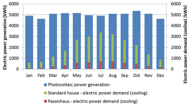
Figure 6-1: Monthly sums of the electric power requirement for the building cooling system as well as the photovoltaic electric power generation
