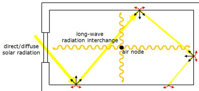
Figure 2-2: Schematic representation of the calculation of solar irradiation distribution and heat radiation exchange in the interior
