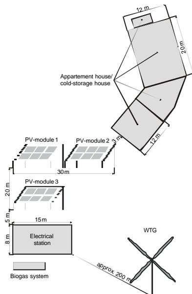
**Fig. 3:** Arrangement of VATALI’s main parts.
