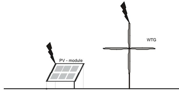
**Fig. 4:** Integrated LPS with direct strikes to the components (here: PV-module and small WTG).
