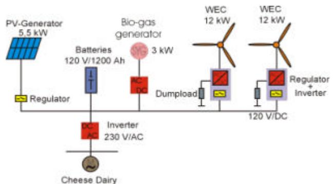
Fig. 2: Schematic diagram of the hybrid-system VATALI (extract).
