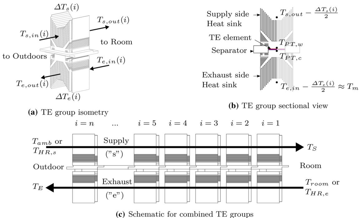
Fig. 1 Schematic system design
