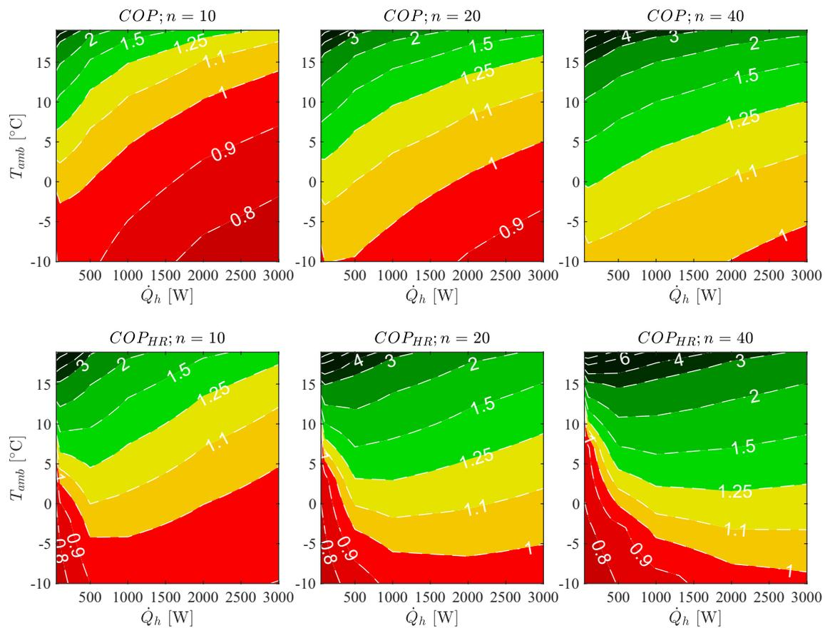
**Fig. 7** Coefficient of performance for various ambient temperatures  $T_{amb}$  and various heating demands  $\dot{Q}_h$  at  $n = [10, 20, 40]$ . Top: without heat recovery unit. Bottom: with heat recovery unit
