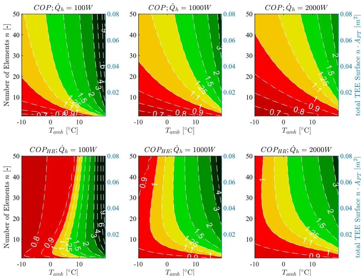
**Fig. 3** Coefficient of performance for various numbers of TEEs, various ambient temperatures  $T_{amb}$  at a total heating demand of  $\dot{Q}_h = [100W, 1000W, 2000W]$  Top: no heat recovery unit. Bottom: with heat recovery unit
