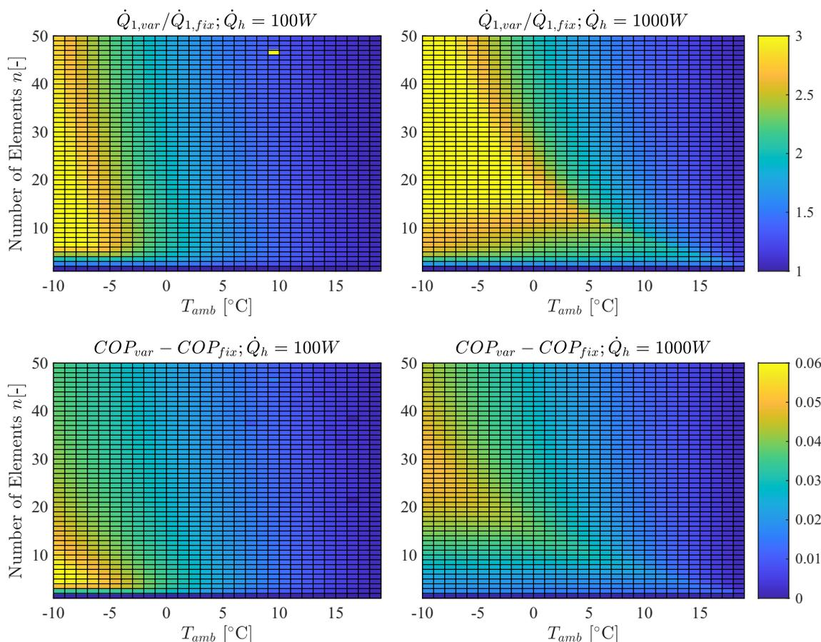
**Fig. 6** Top: Heating load at roomside TEE of the supply stream for uneven heat distribution  $\dot{Q}_{h,1,var}$  related to heating demand at even heat distribution  $\dot{Q}_{h,1,fix}$  for various numbers of TEE, various ambient
