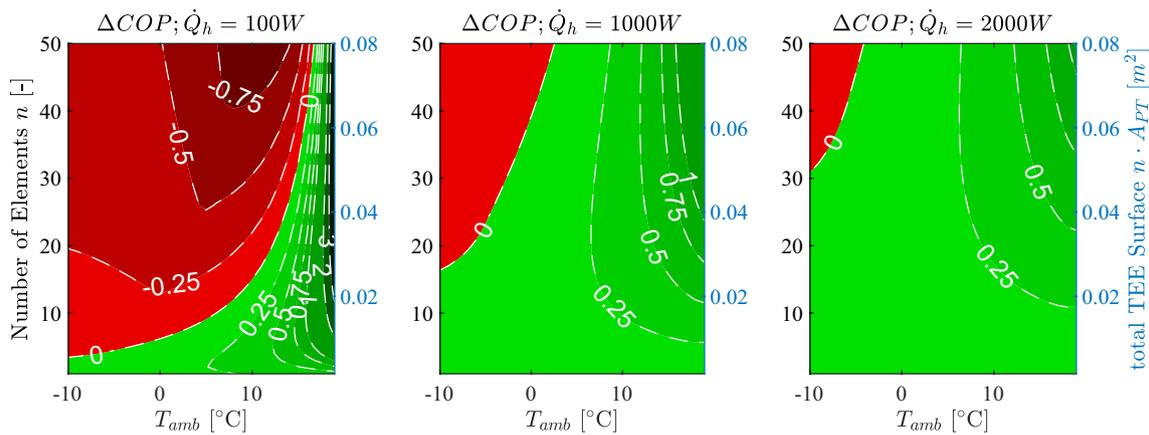
**Fig. 4** Change in the coefficient of performance due to the use of an upstream heat recovery unit for various numbers of TEEs, various ambient temperatures  $T_{amb}$  at a total heating demand of  $\dot{Q}_h = [100W, 1000W, 2000W]$
