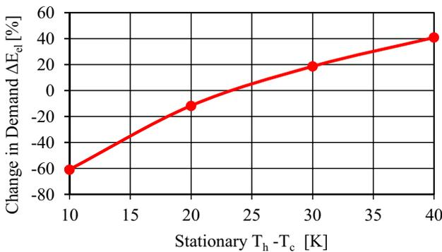
**Fig. 5** Estimation of change in calculated electrical energy demand  $\Delta E_{el}$  for transient simulation instead of the steady state simplification for one TEE
