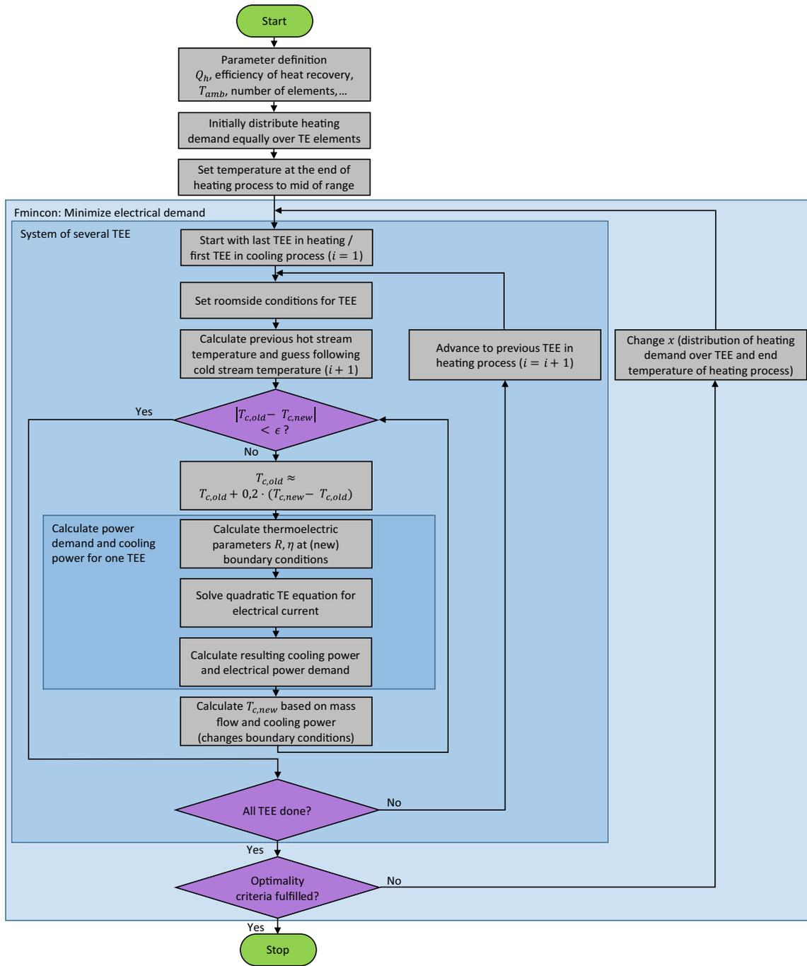
Fig. 2 Flow chart containing the main operations of the optimization process
